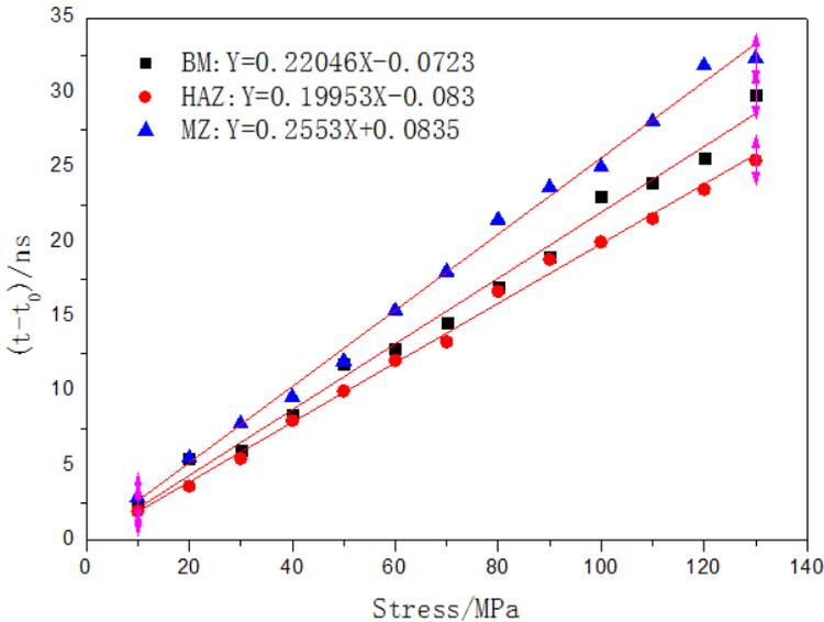
Fig. 7. (Color online) Result of tensile test to evaluate the  $K$ .
