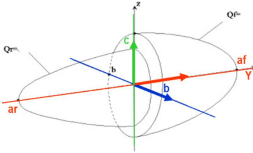
Fig. 2. (Color online) Double ellipsoid heat source model.
