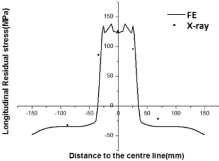
Fig. 10. The comparison of FE method and X-ray method according to residual stress.
