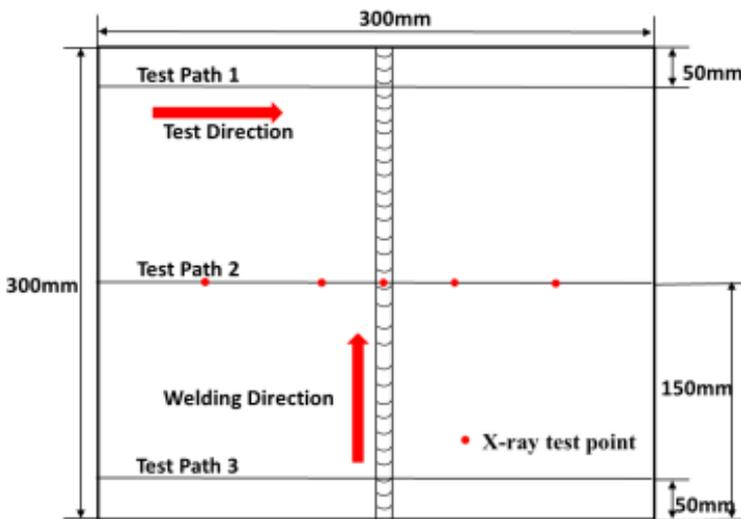
Fig. 9. (Color online) Path of distribution of LCR wave measurement and X-ray resting points.
