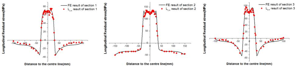
Fig. 12. (Color online) The compare of FE and LCR method of residual stress results in different testing path.
