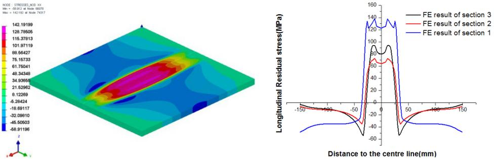
Fig. 11. (Color online) Longitudinal residual stress results of contour and three sections.
