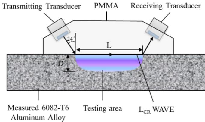
Fig. 5. (Color online) LCR wave testing device.
